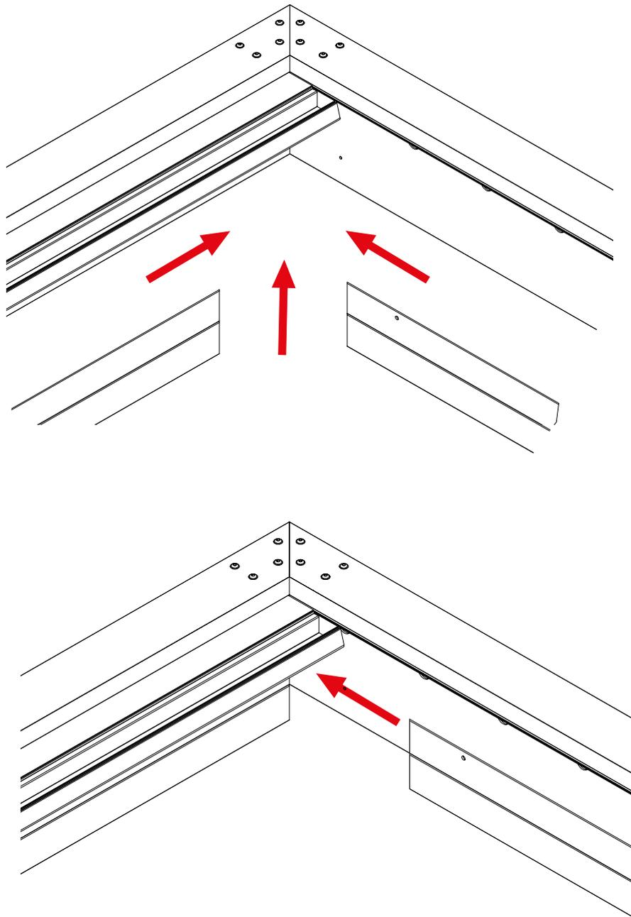
Check that all the "U" profile holes match the M6 machined ones on the beam. If all match, apply sealant between the U-profile and the beam and around the screw holes, then screw the profiles together using ULS (ISO 7380) A2 M6x16 screws.
